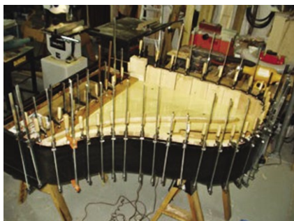
Gluing a new soundboard into the rim of a grand piano
