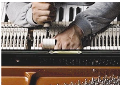
Custom voicing of a piano for optimal tonal quality is considered by piano technicians to be an art form.
