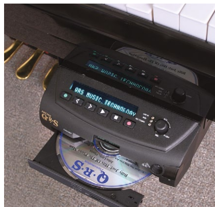
The QRS Pianomation Ancho controller includes CD and Compact-Flash drives.
