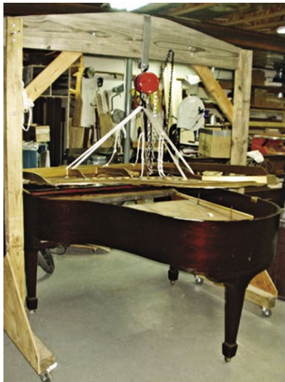
Reinstalling the cast-iron plate during the rebuilding of a grand piano
