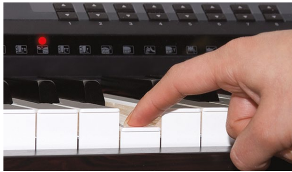
Educational feature: A light indicates to the student which key should be pressed next.
