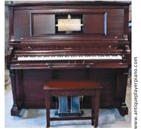
An old-fashioned, pneumatically driven player piano with punched-paper music roll and pumping pedals
