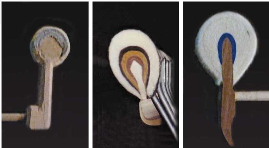
The evolution of the piano hammer: leather-covered hammer, circa 1800; hammer from 1854 Erard, covered in a combination of leather and felt; modern felt-covered Renner hammer.
