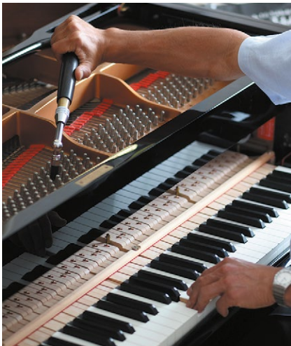
A piano has over 200 strings, each of which must be individually tuned.
