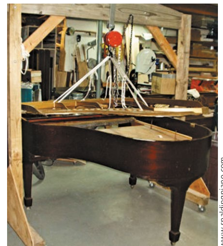
Reinstalling the cast-iron plate during the rebuilding of a grand piano
