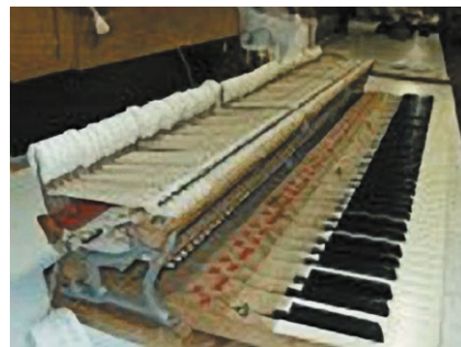
A rebuilt grand piano action with new hammers is ready for regulating and voicing.
