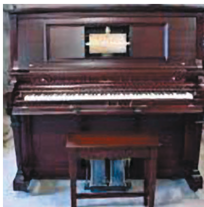
An old-fashioned, pneumatically driven player piano with punched-paper music roll and pumping pedals
