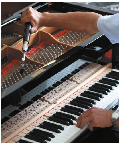
A piano has over 200 strings, each of which must be individually tuned.
