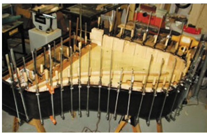
Gluing a new soundboard into the rim of a grand piano
